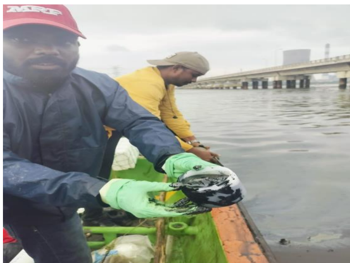
Figure 19: Sediment sample collection from midstream and banks
