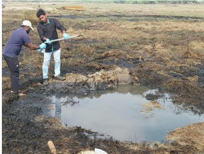
Figure 22: Collecting water samples using a bailer
