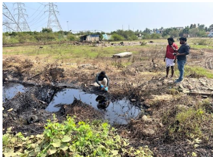
Figure 6: Collection of samples from the oil overflow along the banks of B Canal.
