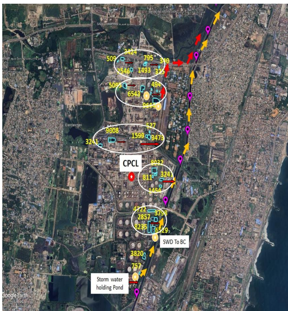
Figure 34: Open tank locations and area in sq.m.
